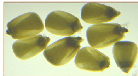
Stress cracks present in corn
